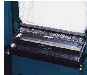
MVW Units house a 4" Chevron Impinger, 1" Aluminum Mesh and 36" Vee Bag filter
